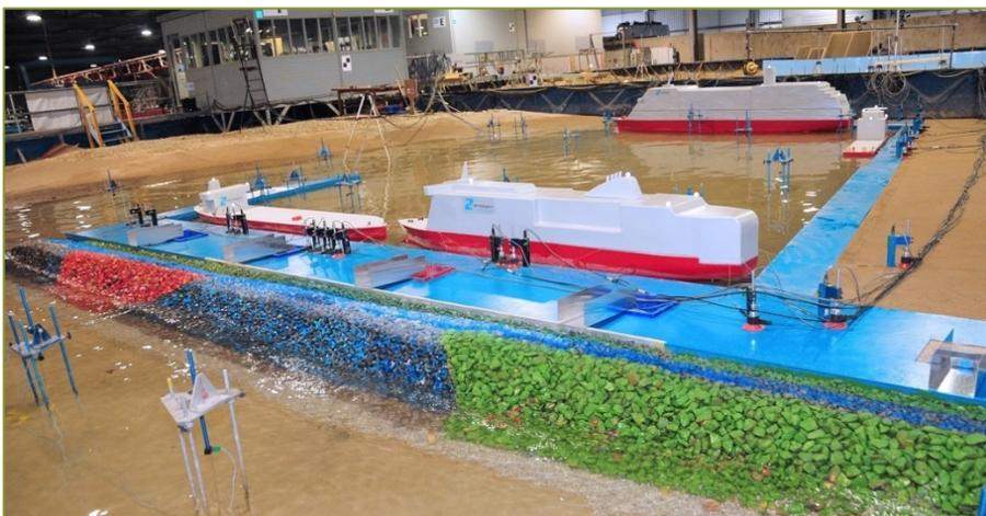
To ensure ships can safely access ports in stormy conditions, the layout can be tested as physical models in laboratories – as pictured above at HR Wallingford.
