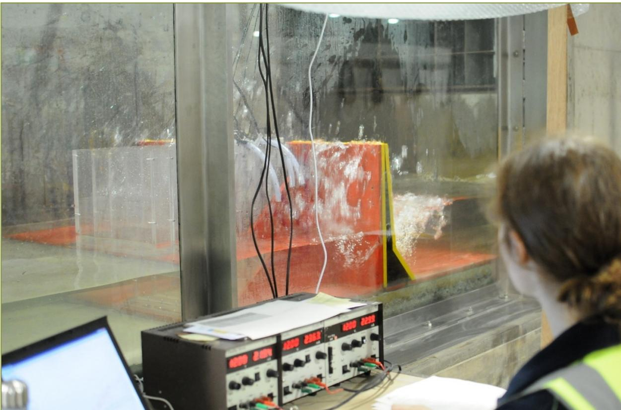
A multi-segmented collection tank measuring the effect of wind on wave overtopping was developed for the WindWave project. HR Wallingford, which was part of the National Environment Research Council (NERC)-funded research consortium, tested different wind speeds using the flumes in its modelling hall.
