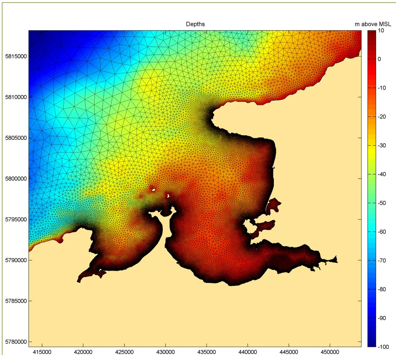
Images generated of Tralee and adjacent bays in south-west Ireland by HR Wallingford using a calibrated tide, surge and wave forecast system, which could be used as an indicator of potential coastal flooding.
